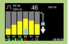
overall measurement can be stored in the device and displayed on a map on the PC using the HydroluxView software. The stored leak noise can be played back with just a mouse click.
