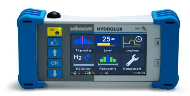
Thanks to the integrated Bluetooth<sup>®</sup> technology, there are no more interfering cables between the operating unit, the headphones and the respective sensors. Interfering noise caused by the wind or cable contact is a thing of the past. You can therefore devote your full concentration to the leak noise.
